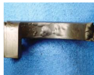
Elastomer seals affected by explosive decompression.
