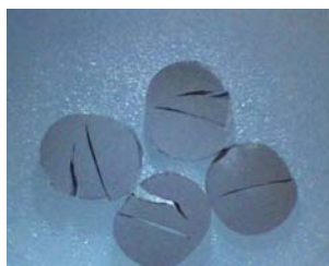
Elastomer seals affected by explosive decompression.
